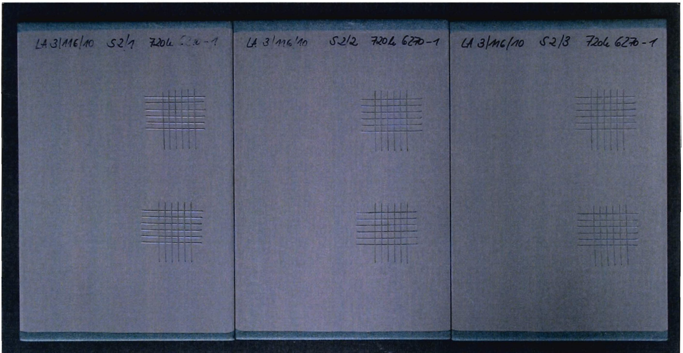
Fig. 1: test specimens after loading with condensation of water
